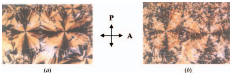
Figure 10. Photomicrographs showing (a) the racemic ferroelectric state obtained in the B_{2X} phase of compound 16 by application of a d.c. field ( \pm 10 \text{ V } \mu\text{m}^{-1} ), and (b) the texture obtained on turning off the electric field, indicating the racemic nature of the domains. Note that the dark brushes obtained exist along the directions of the crossed polarizers.
